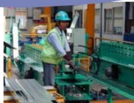
Truss components are manufactured
